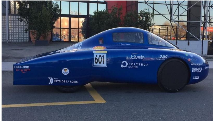
Figure 6 Example streamlined prototype (CityJoule 2 hydrogen car) with very low drag design. Its shape resembles a boat-tail configuration minimizing the wake.
